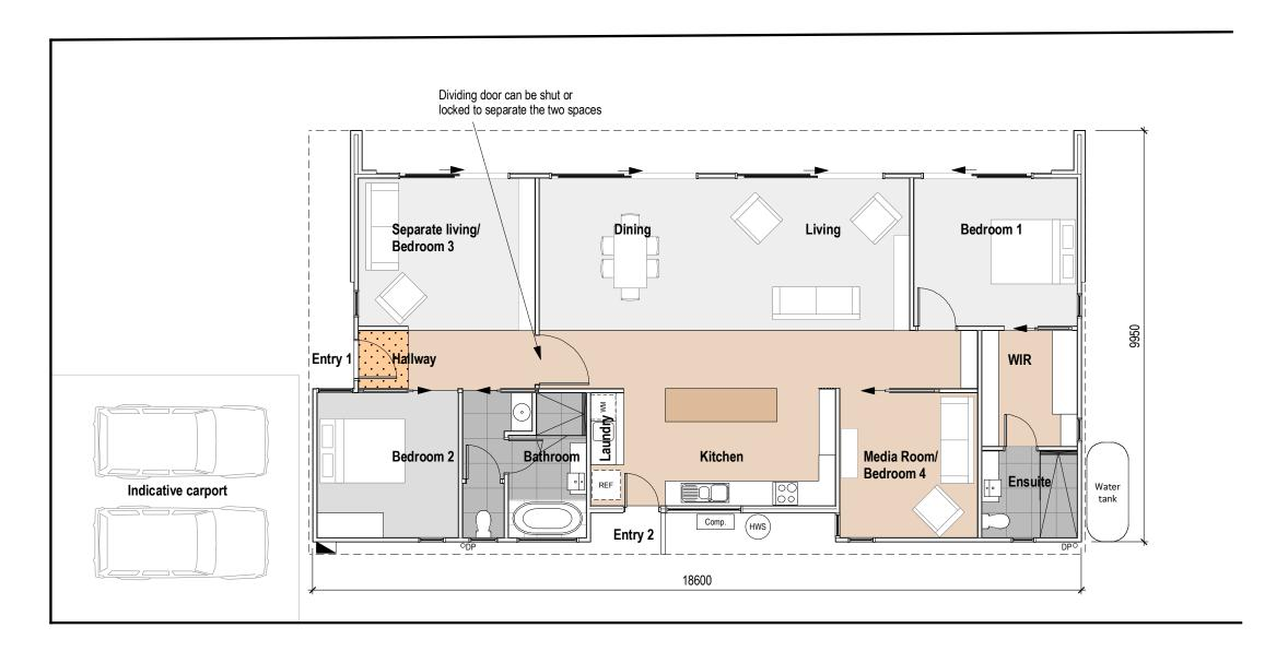
Energy Efficient Demonstration Home - Floor Plan: multi-generational living option 2b - 156sqm Scale 1:100 on A3
